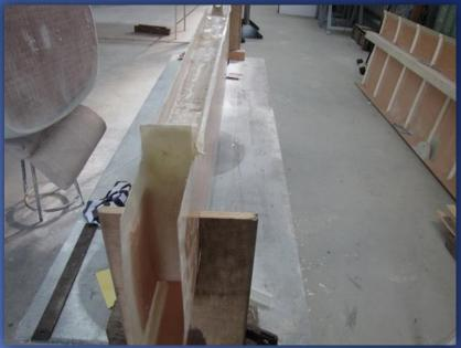
The reinforcement for the hinge point elevator is glued in and glassed over.
