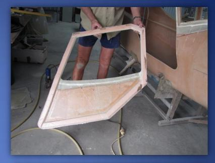
The doors are trimmed and later refitted into the installed door frames.
