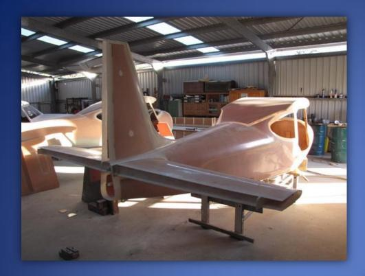
Horizontal tail plane is set into position ready to be glued and glassed in.
