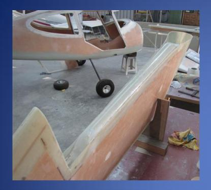
The rudder is installed into its hinge socket and the control mechanism adjusted for correct movement and length
