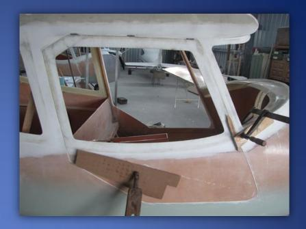
With the door frames glassed in and hinges attached, the easy access upward swinging doors are ready for alignment and fitting.
