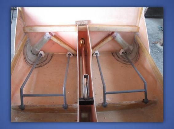
Next, the Control-Arm is fitted into the Centre-Console.
