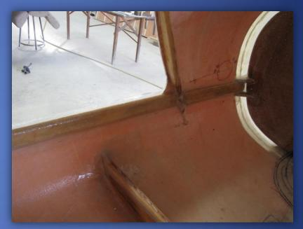
The glassing over method also preserves the material, which it is encasing in the process.
