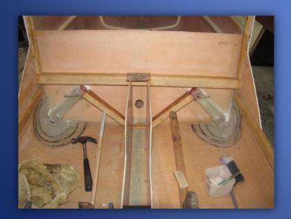
The prefabricated leg bushes are fitted onto the Chrome-Molly legs then glued in situ and glassed over.
