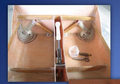
The control stick is then attached to the control arm which is guided through a rocker-mechanism and support-guides through to the rear of the fuselage.
