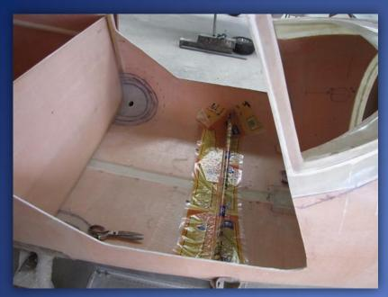
The connecting support brace is glued in and glassed over.
