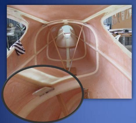
The seat belt attachments are propped into position, glued & glassed in place.
