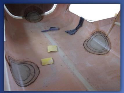
The main & front wheel fuselage protrusion-points are reinforced with 6 extra layers of glass for each leg.
