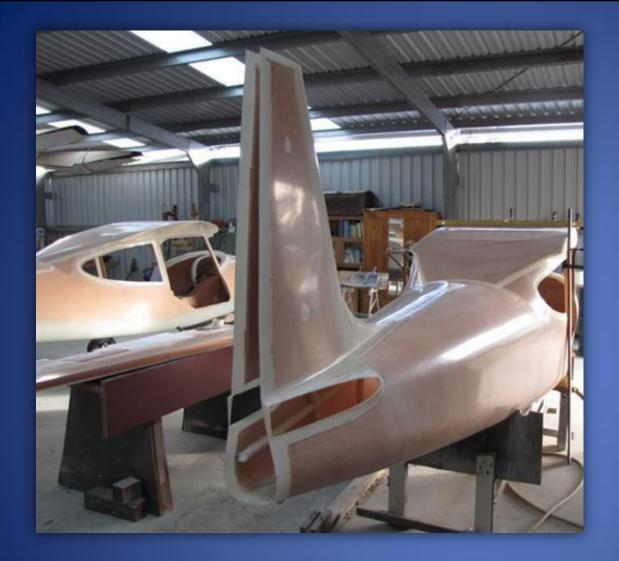
From the vertical tailplane, the rudder is cut-off, leaving the fin. Next, the openings for the horizontal stabiliser are cut-out.
