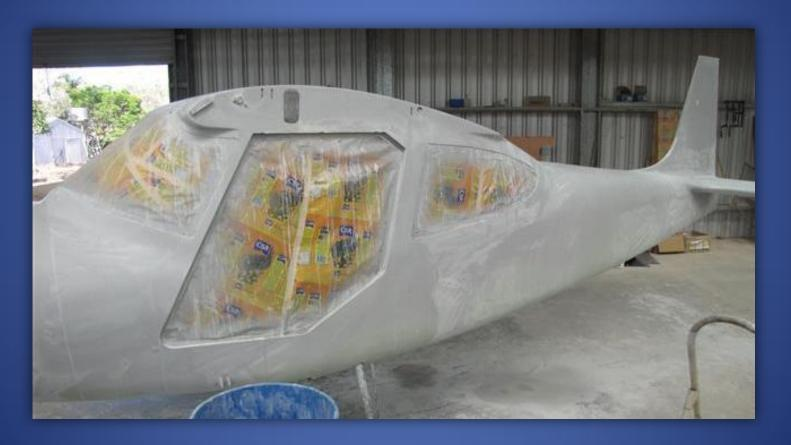
The high strength Polyurethane top coat gives a polished finish.
