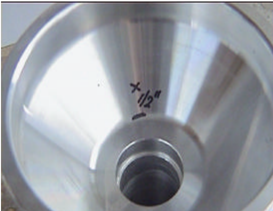
Drill 12mm hole approx. 12mm from edge.
