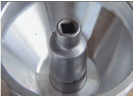
Put pressure just to outside of bearing.
