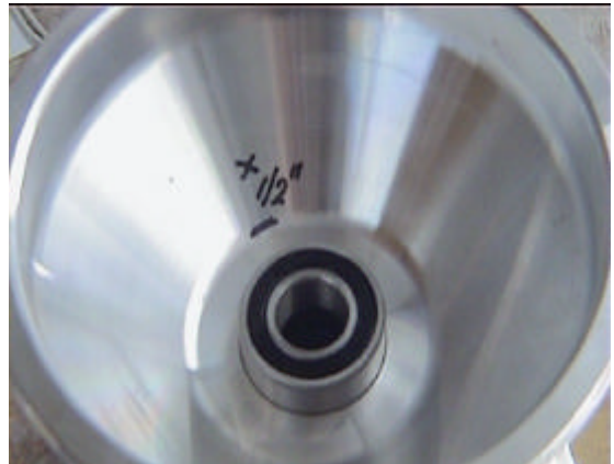
Position bearing ready to press in.
