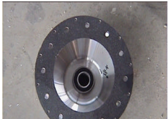
Drill rim, use brake disc as drill jig, rivet disk to rim.
