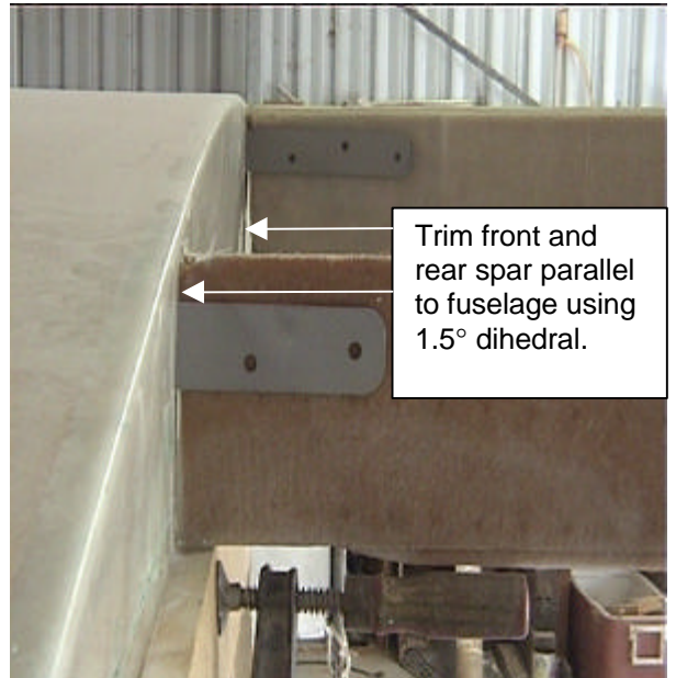
Attach bottom wing to fuselage.
