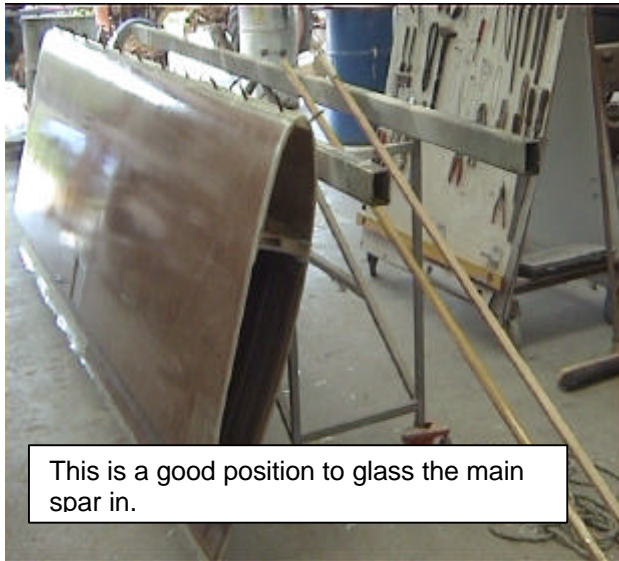
Use a tube or broomstick and wrap it with packing tape and put brush on a long handle.
