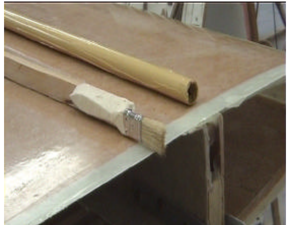
Use a tube or broomstick and wrap it with packing tape and put brush on a long handle.
